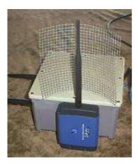
You can make a parable from plain cardboard, or chicken wire. The following web site describes how to build your own parable and has a specific template for use with a WET11: http://www.nodomainname.co.uk/parabolic/parabolic.htm
